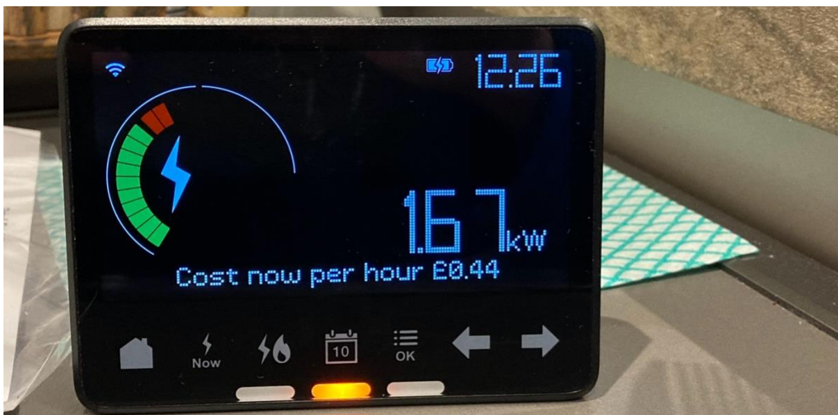
Figure 11: In building display showing current peak demand and current cost per hour
