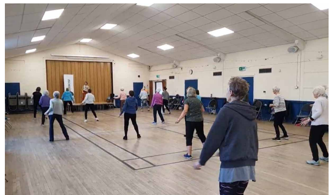
The old ceiling tiles at Haddenham were replaced with sound-absorbing ceiling panels, a very simple and effective way to soften the acoustic
